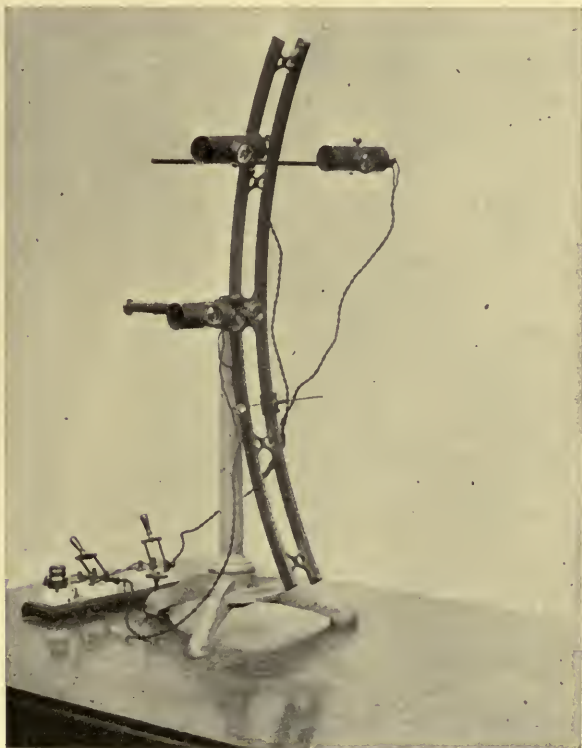
FIG. 56.—Ophthalmophacometer of Tscherning. The arc vertical.
